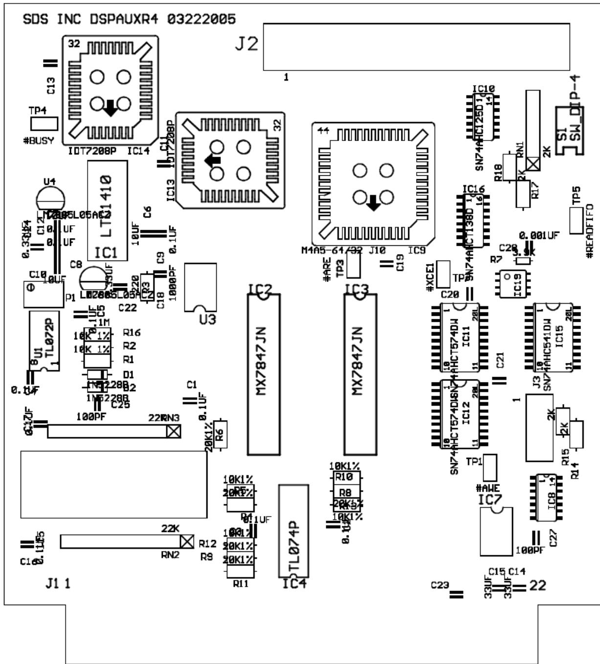
Fig 14.2 DSPAUX R4 board layout
