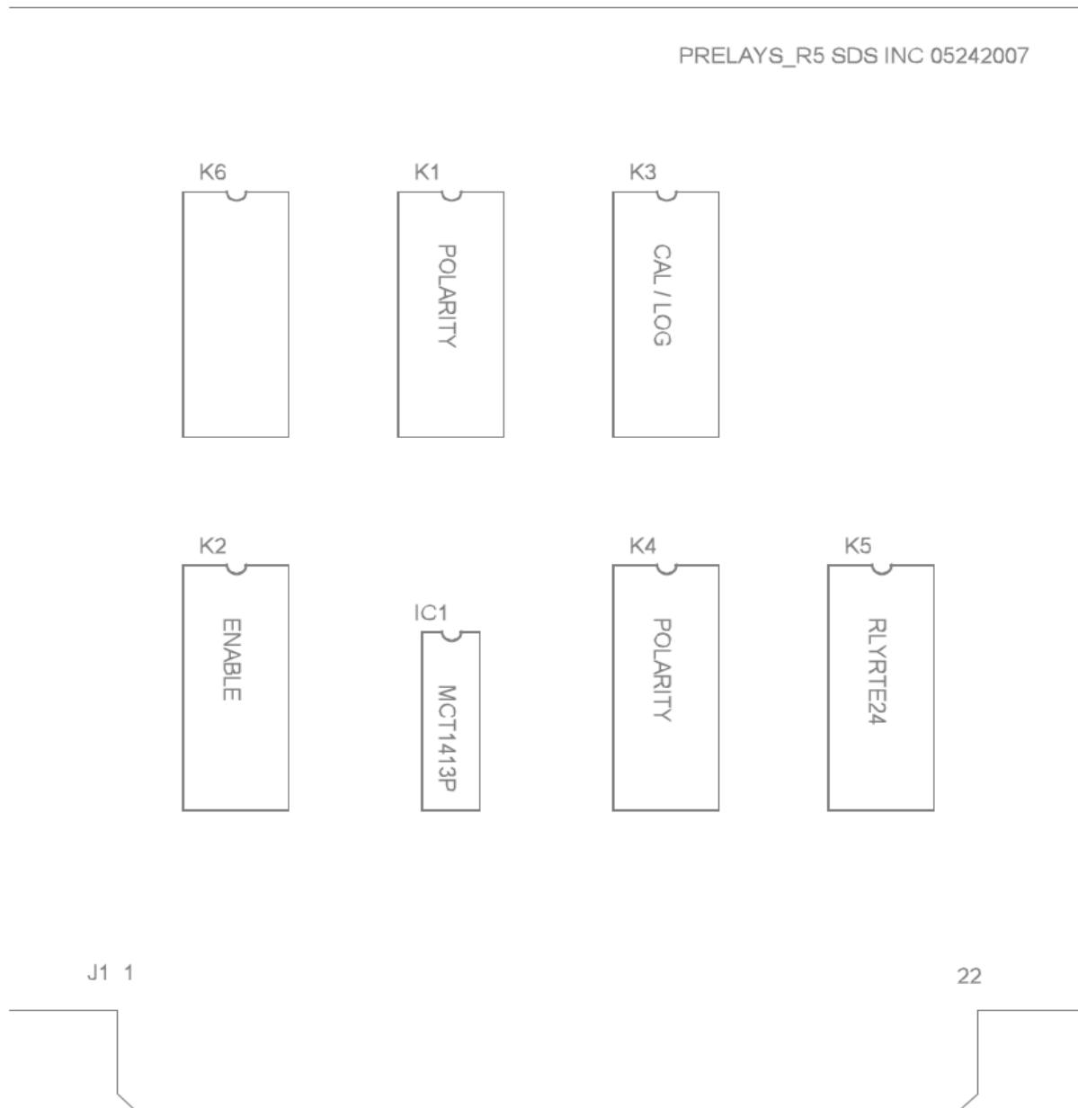
Fig 3.2 Pre-Relay R5 board layout
