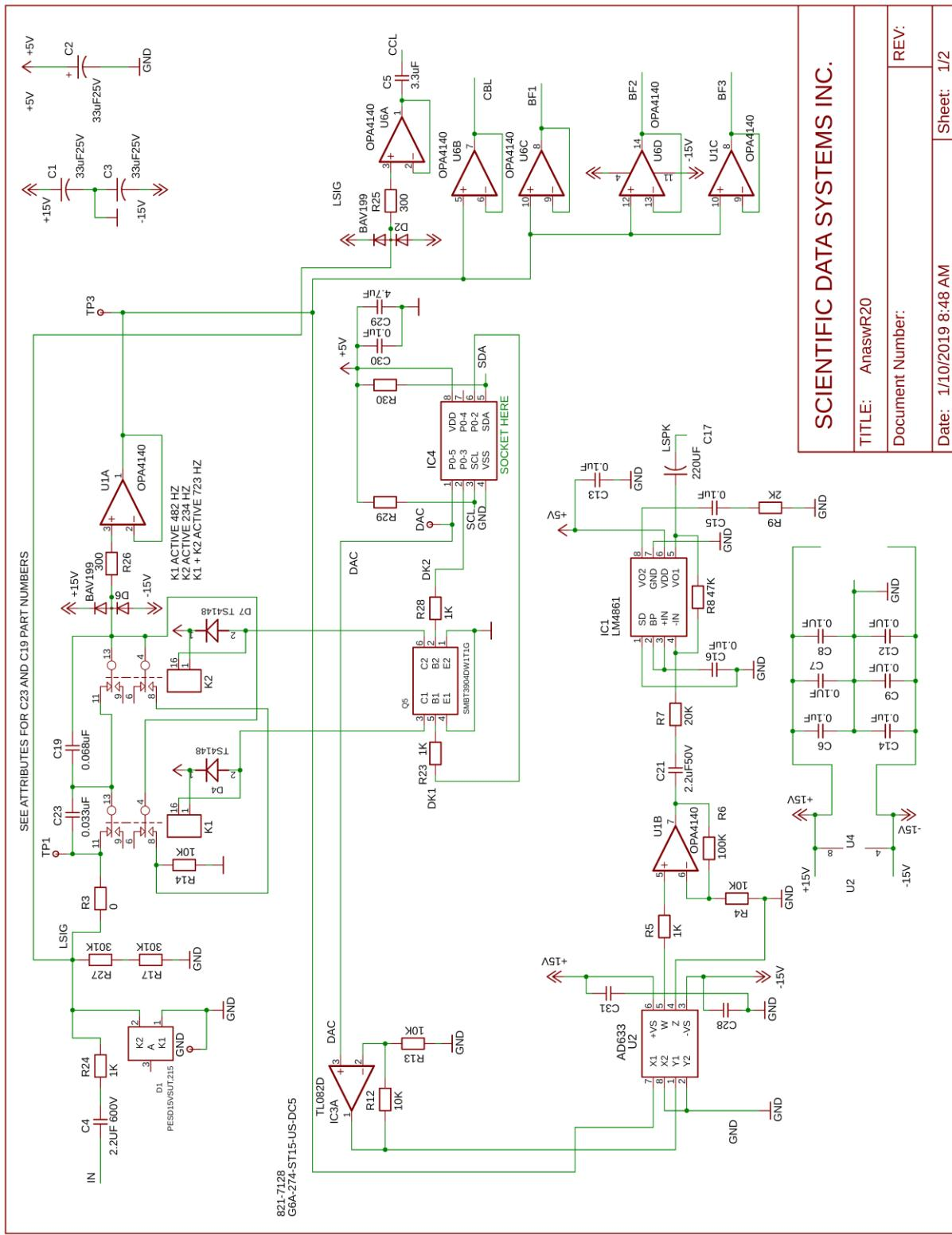
Fig 7ii.1 Schematic Analog Switch ANASW R17
