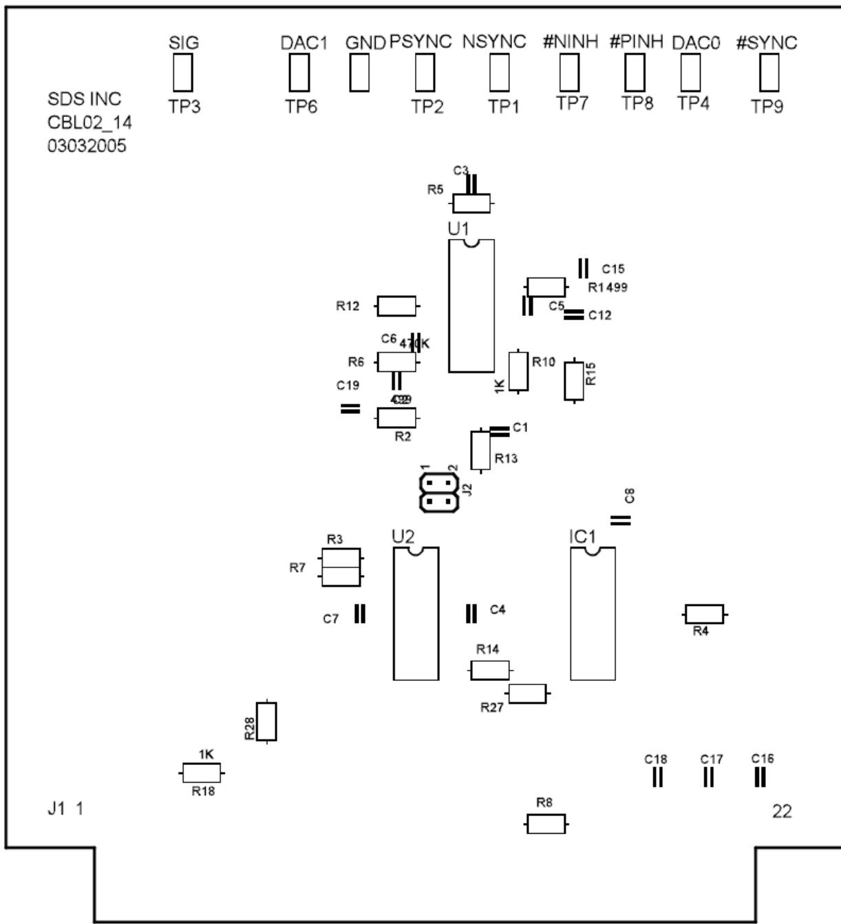
Fig 10.2 CBL2 R14 board layout
