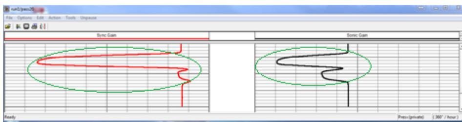
Fig Jii.10 5k -20k Hz frequency sweep Q=2 Band Pass
