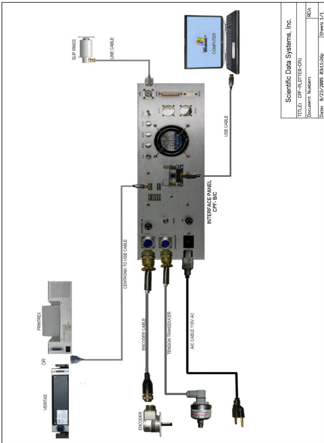
Fig 1.1 CPF-Plotter-CPU
