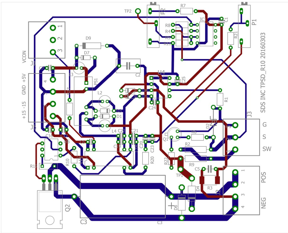
Fig 6.2 TPSD R10 board layout
