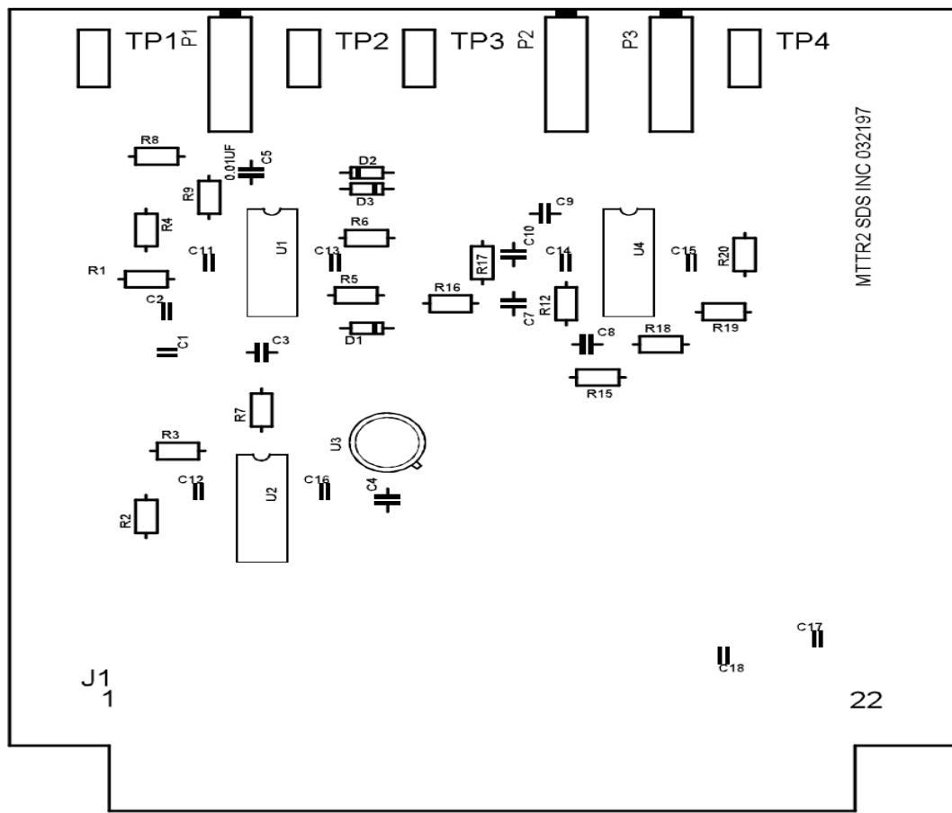
Fig 12.1 MTT R2 board layout
