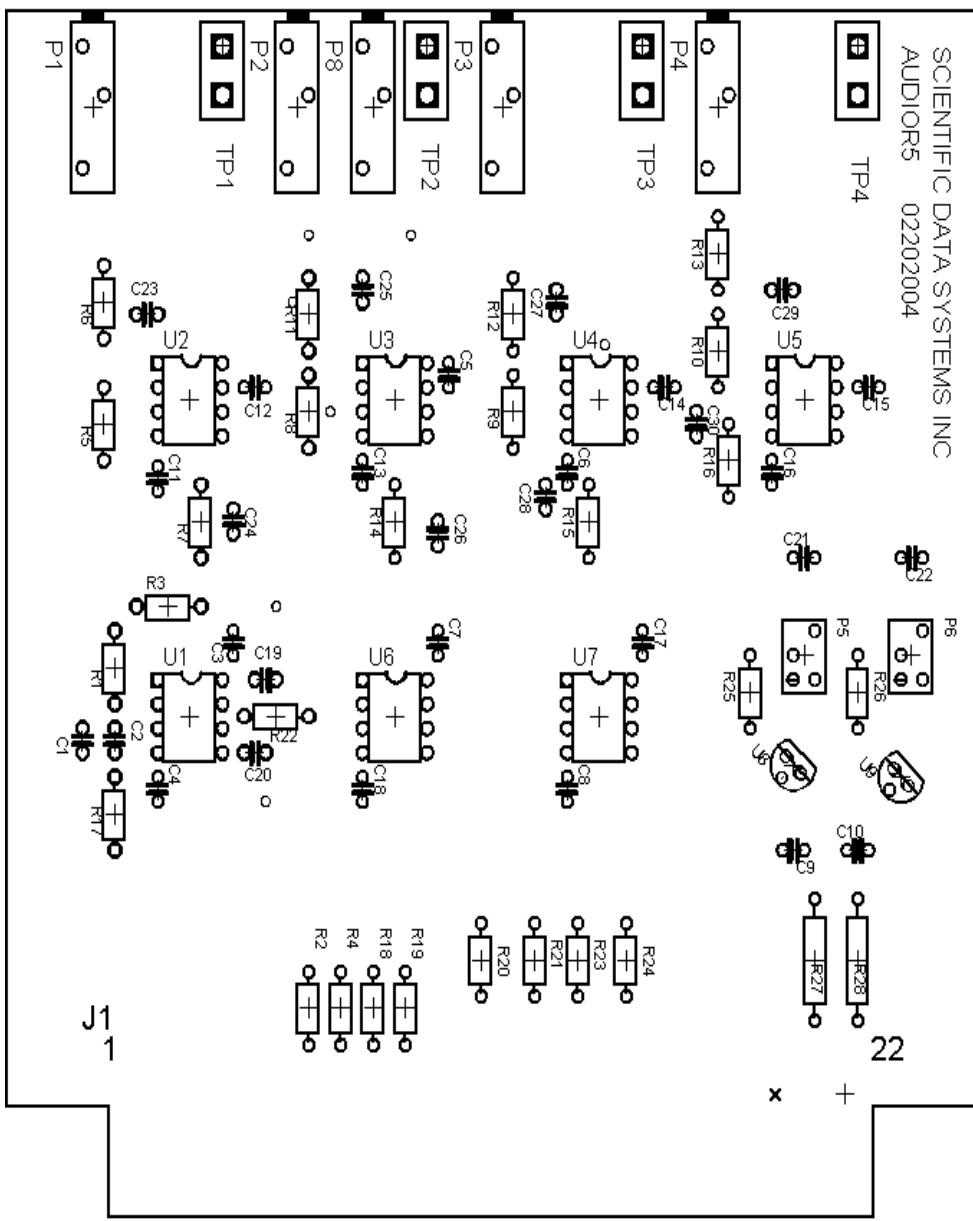
Fig 11.2 Audio Board R5 board layout
