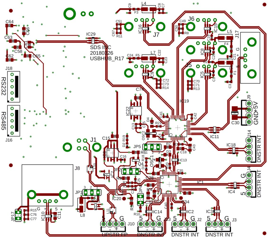
Fig 16.2 USB2 R18 Hub board layout
