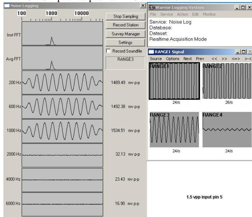
Fig. L.4 1 KHz @ 1.5 vpp at Pin 5 the Audio Board
