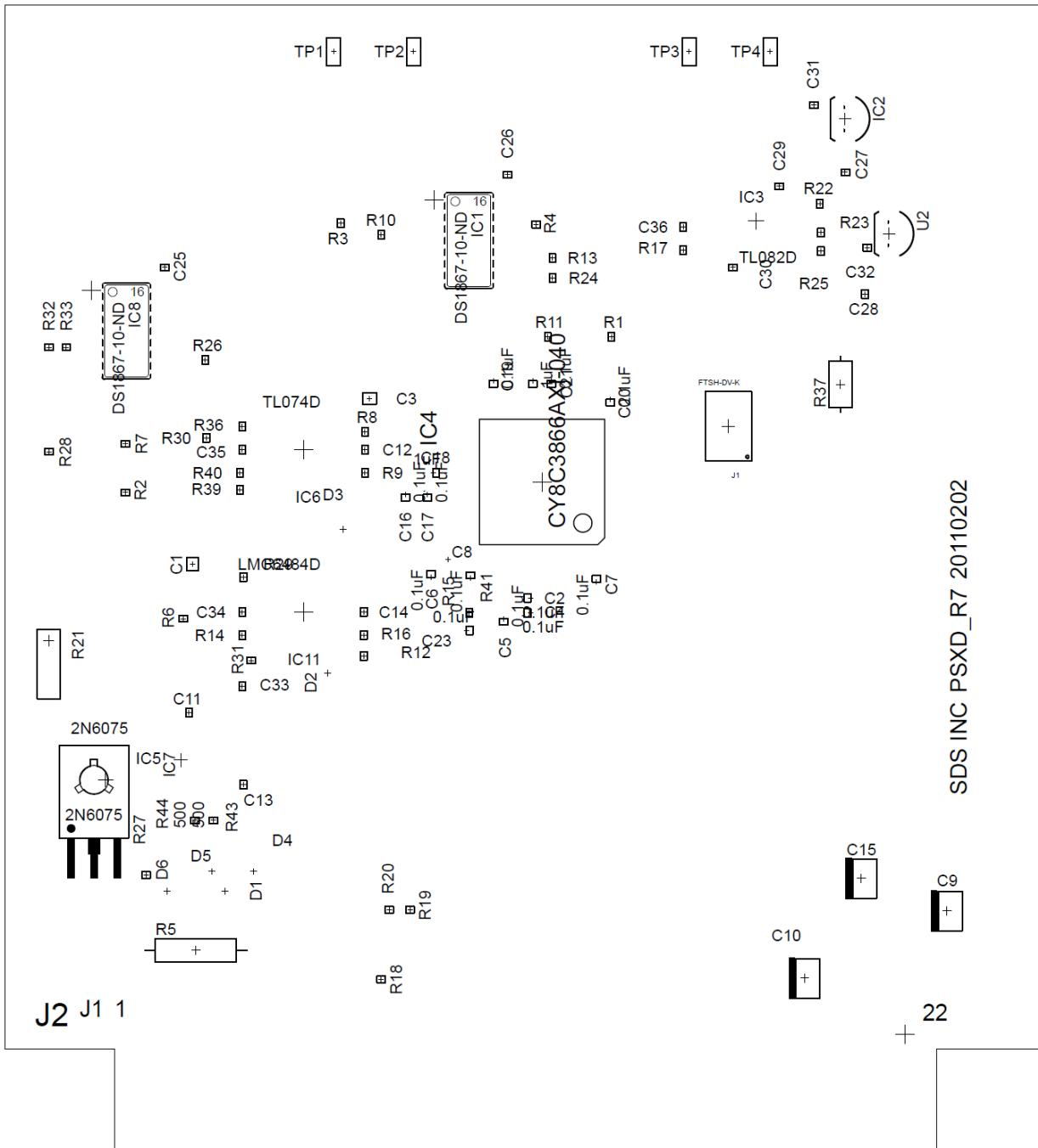
Fig 5.2 PSXD R7 board layout
