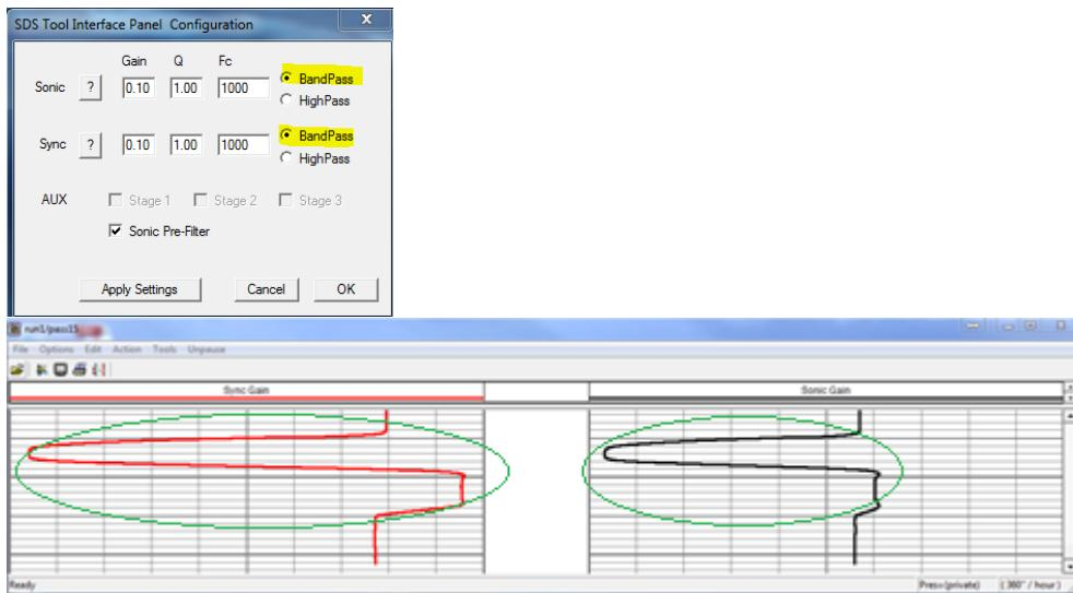
Fig Jii.6 200-2k Hz frequency sweep Q=1 Band Pass
