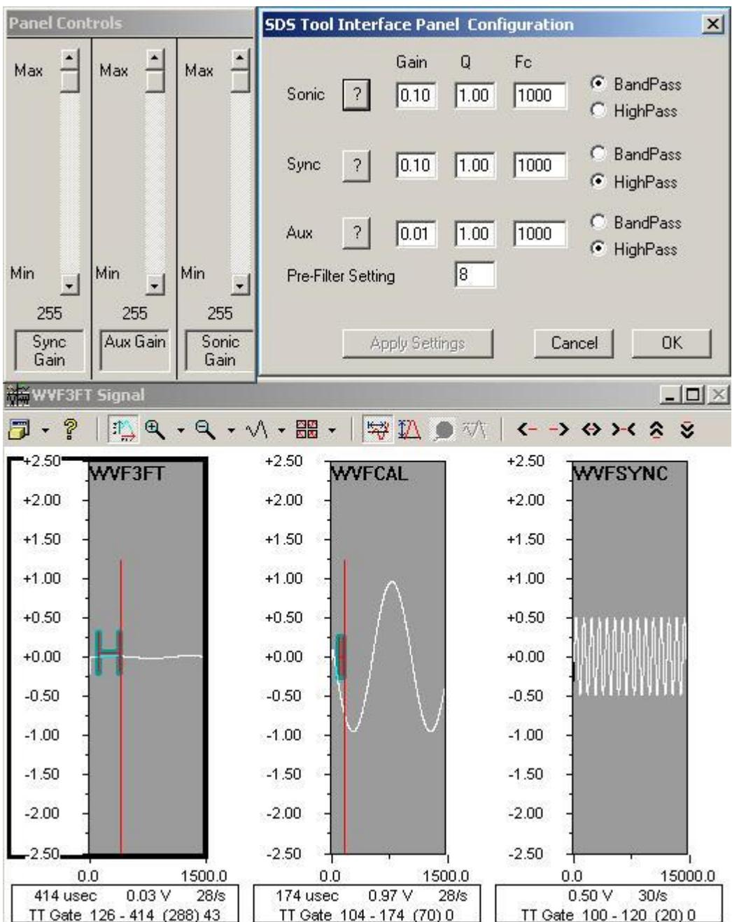
Fig. Ji.16 CBL1-Test Service 1Khz .5Vpp Pre Filter Setting 8
