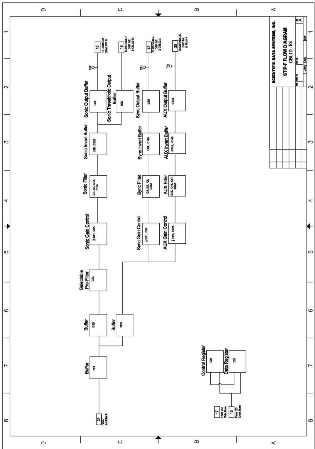
Fig 9i.1 Block Diagram CBL1D R6
