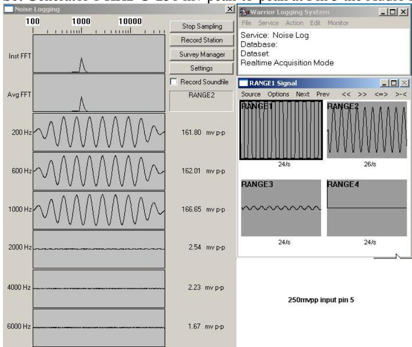
Fig. L.3 1 KHz @ 250 mvpp at Pin 5 the Audio Board
