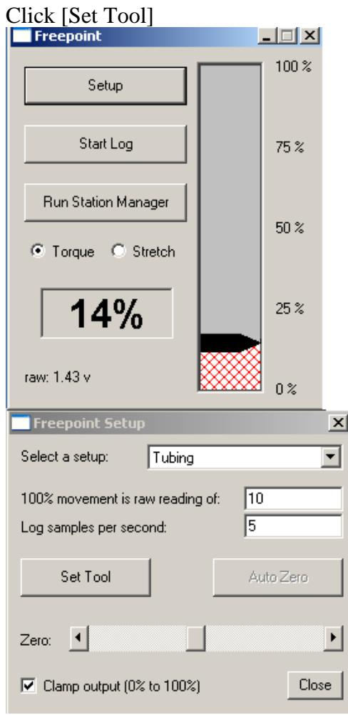
Fig. M.2 Freepoint Adjustment
