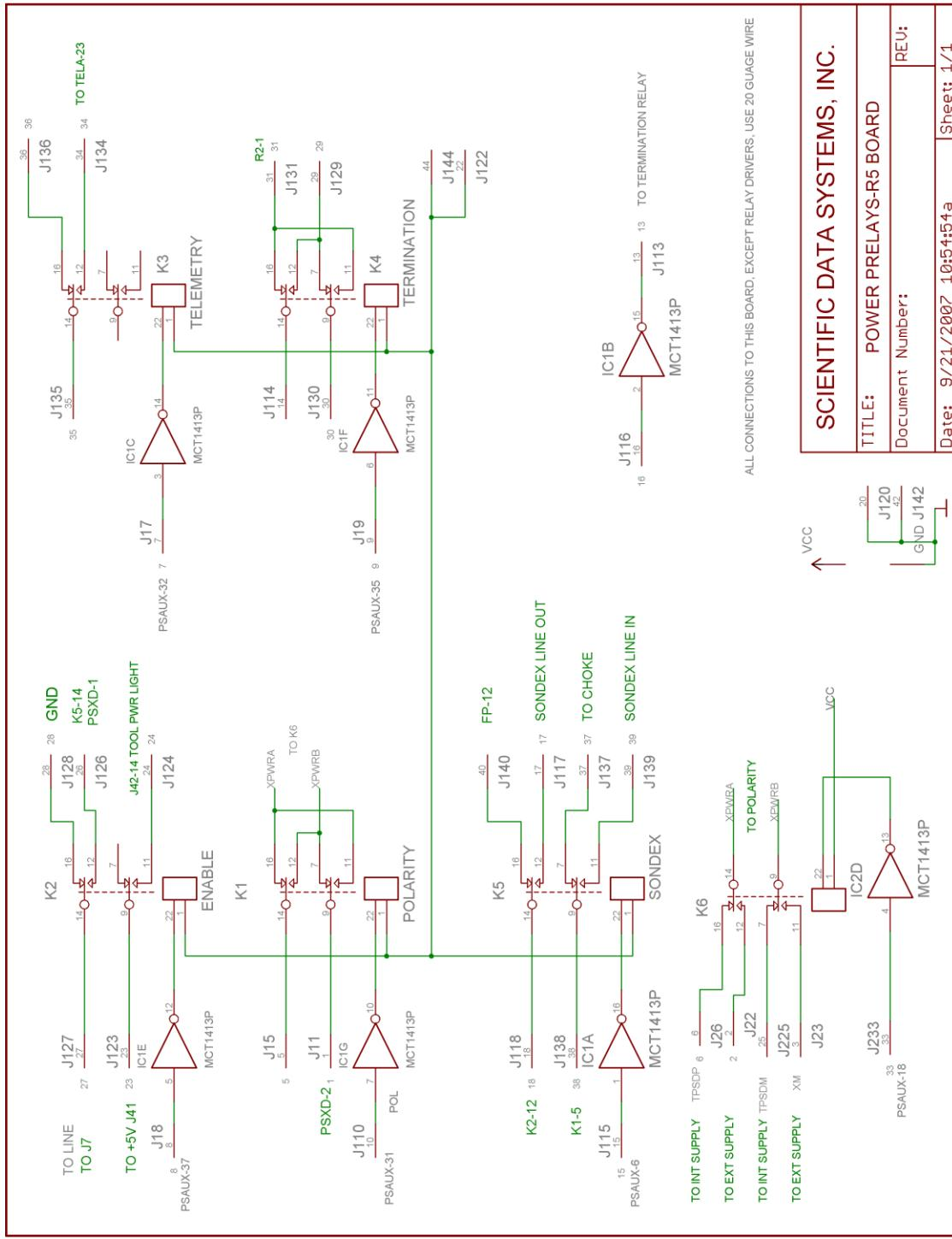
Fig 3.1 schematic Prerelay R5
