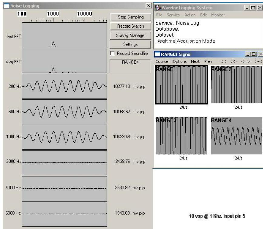
Fig. L.4 1 KHz @ 10vpp at Pin 5 the Audio Board
