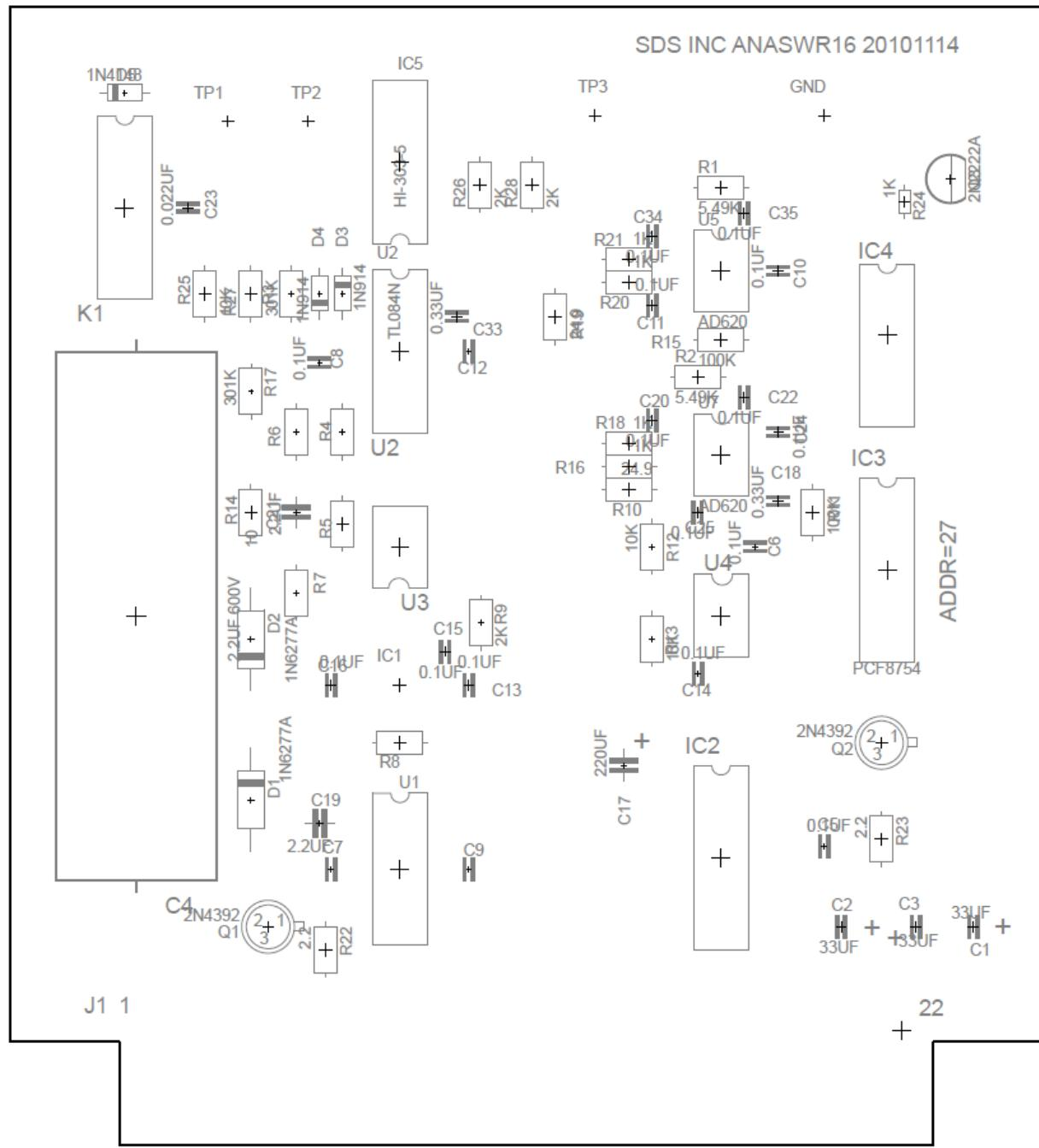
Fig 7i.2 Analog Switch ANASW R16 board layout
