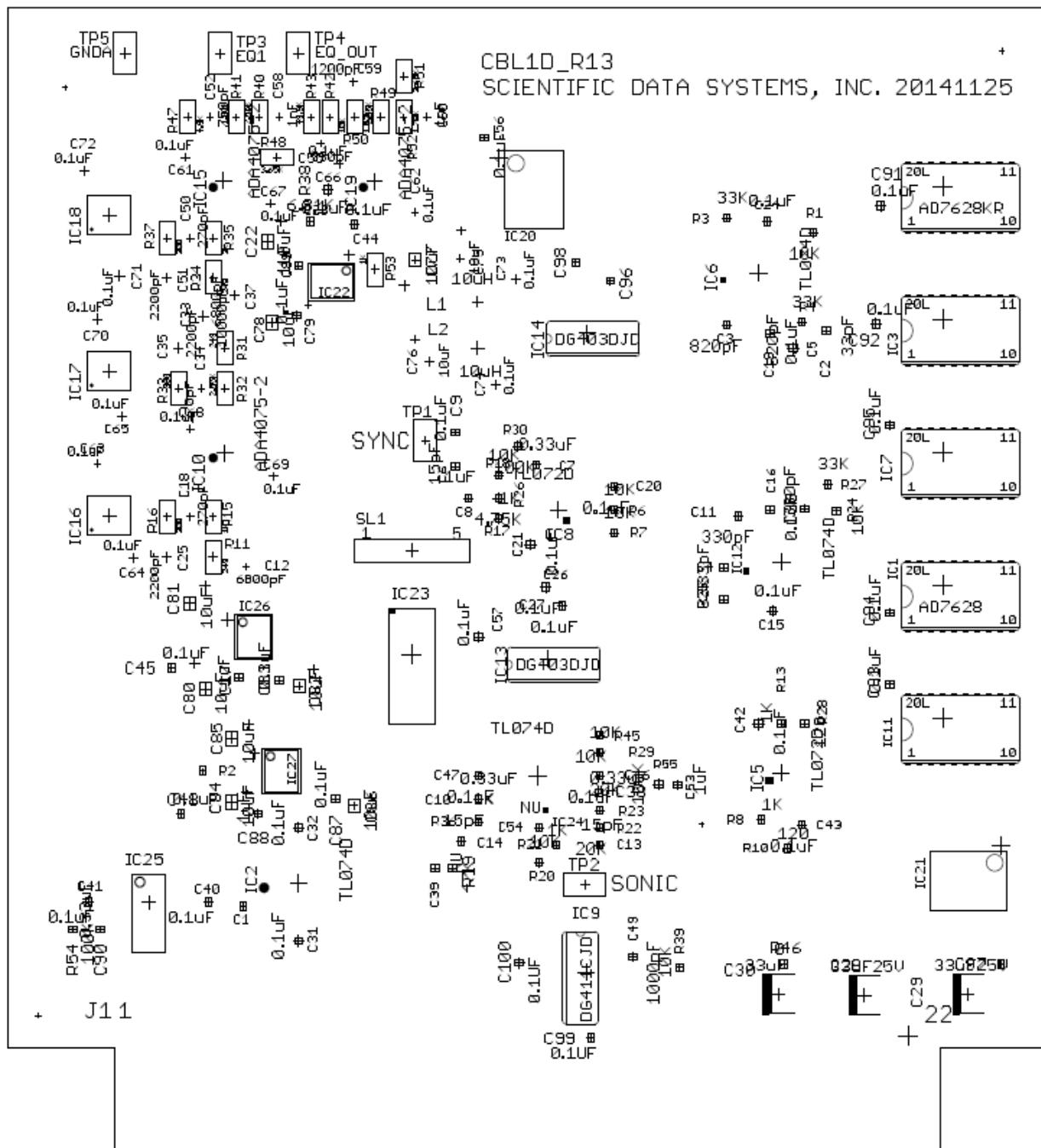
Fig 9ii.3 CBL1 R13 board layout
