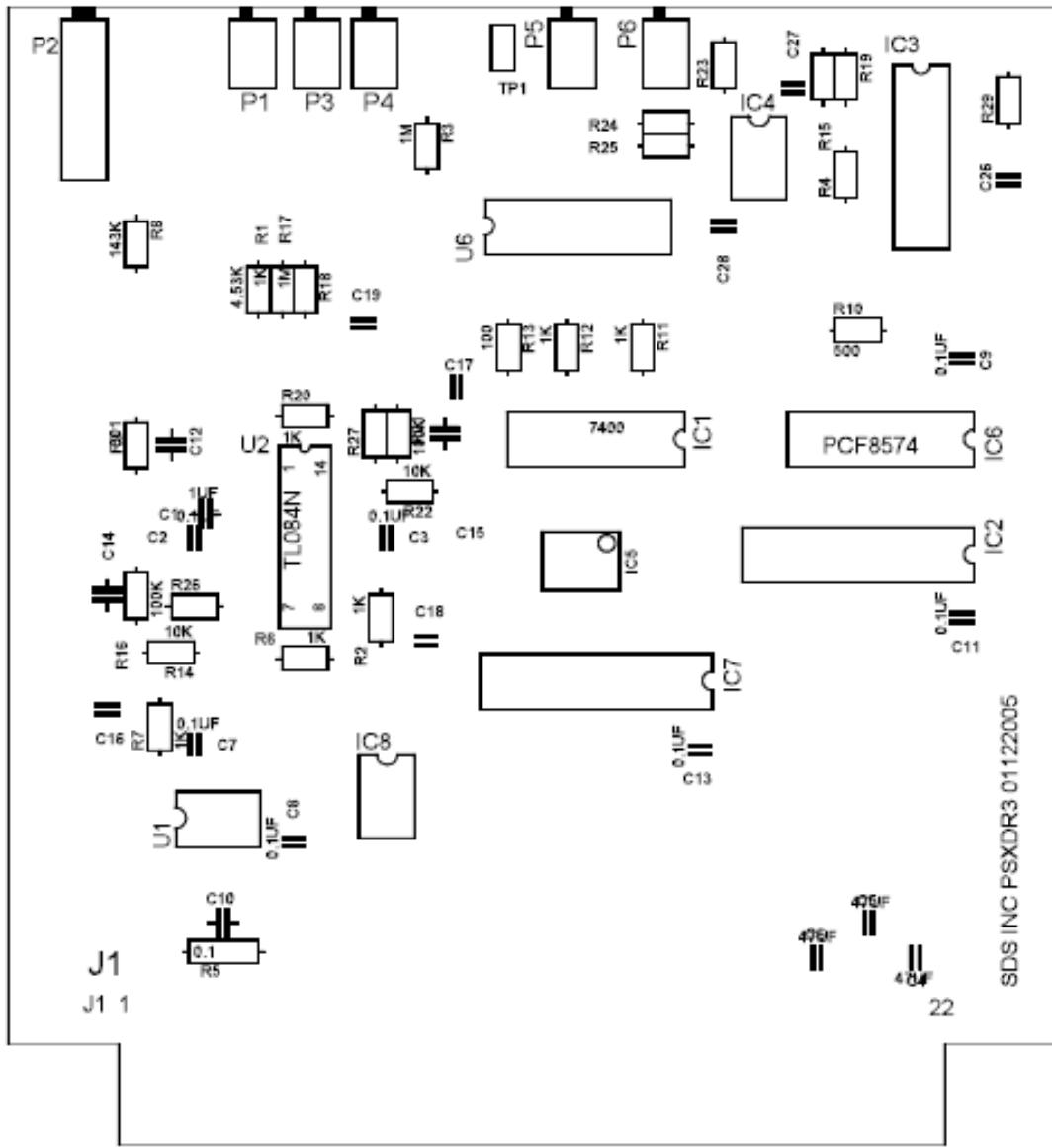
Fig 5.4 PSXD R2 board layout
