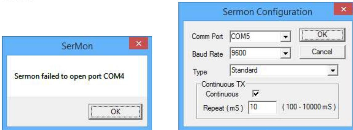
Fig 34.2 Sermon port failed to initialize and Sermon COM port settings.
