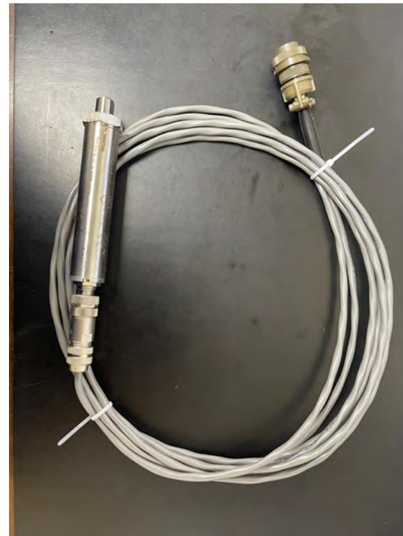
Dyer pressure transducer with custom cable can provide a surface tension readings on all SDS data acquisition systems when used with a hydraulic bellows type tension gauge. The series 626 transducer is a intrinsically safe 4-20ma 500 psi transducer. It has a 1/4" MNPT threaded connection and a M-12 4-pin connector electrical interface.
