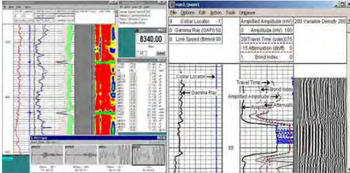
In example shown above, the operator is able to monitor the real time scrolling log, view any or all of the acoustic signals generated by a bond tool, and also monitor all the log outputs, including depth and line speed. Optionally raw sensor data may be displayed.
