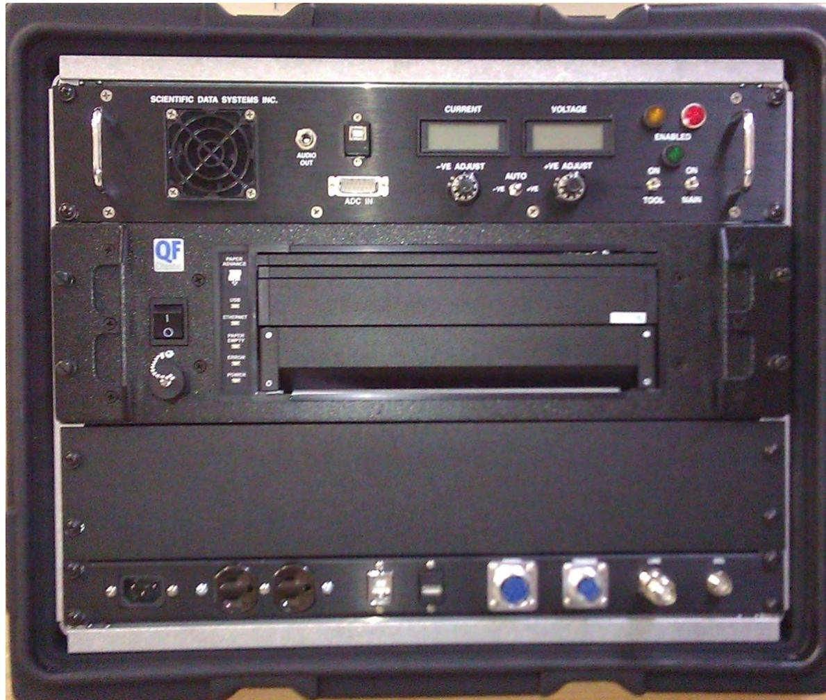
This example shows a PIP panel and Printrex Plotter mounted in a 8u portable rack. There is a 1u interface which brings all the necessary connections to the front of the panel for easy interface with the wireline, surface tension and logging system. A full range of sizes and configurations are available to meet your particular needs.
