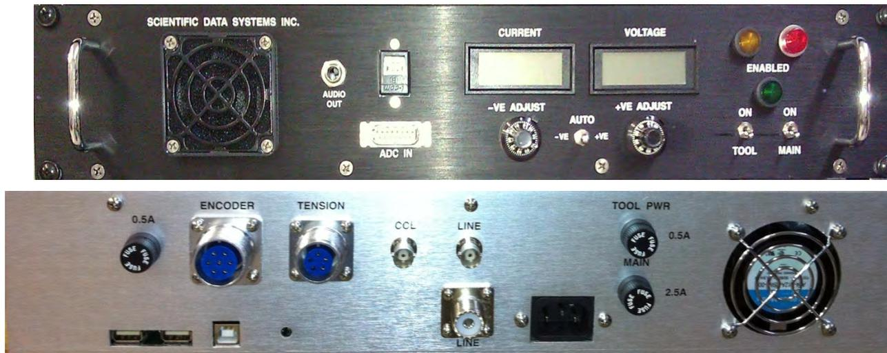
The Pulse Interface panel is intended for use where all the capabilities of the Standard Interface Panel are not required. It is compatible with most pulse based logging tools.
