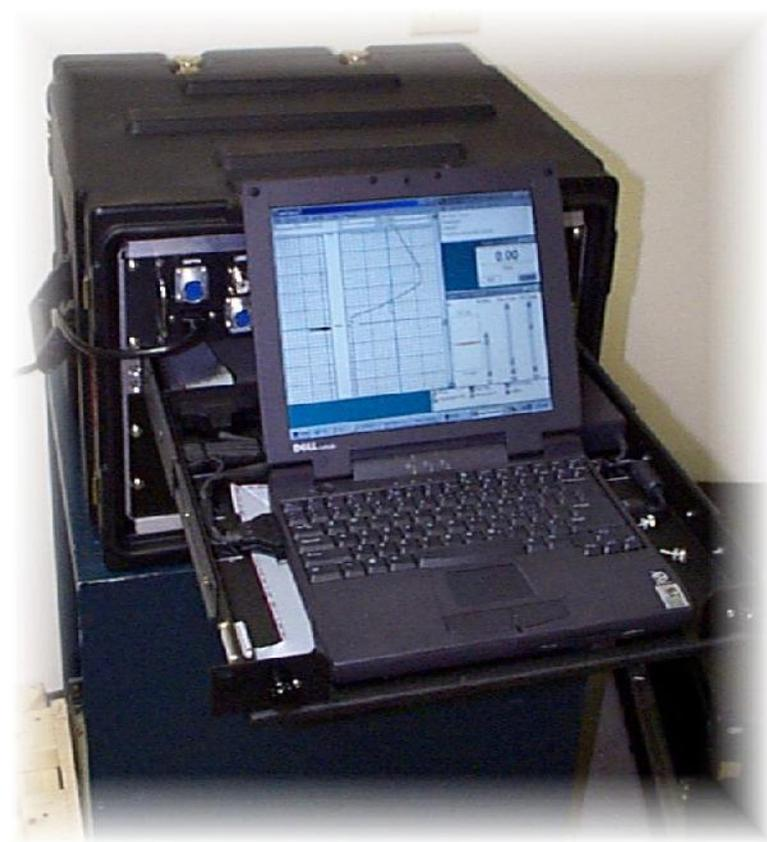
The system supports most downhole tools using pulse type data transmission. It also includes a connector for input of analog signals allowing the system to be used as a data recorder.
