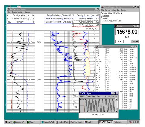
In the example shown at the left the operator is able to monitor the real time scrolling log, view any or all of the acoustic signals generated by an acoustic tool, and also monitor all the log outputs, including depth and line speed. Optionally raw sensor data may be displayed.
