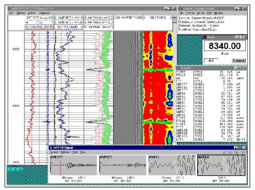
In the example shown at the left the operator is able to monitor the real time scrolling log, view any or all of the acoustic signals generated by a bond tool, and also monitor all the log outputs, including depth and line speed. Optionally raw sensor data may be displayed.
